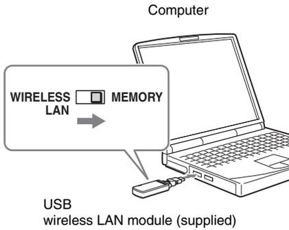
The USB wireless LAN module contains memory. You can switch the built-in memory and wireless connection with the slide switch. To install the Projector Station for Air Shot Version 2, slide the switch to MEMORY. To use the wireless connection, slide it to WIRELESS LAN.
